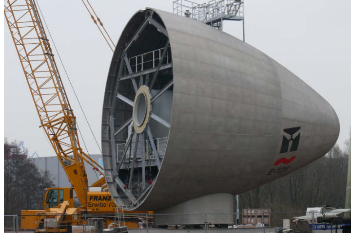
Figure 2-7: Enercon E-126 nacelle [33]
