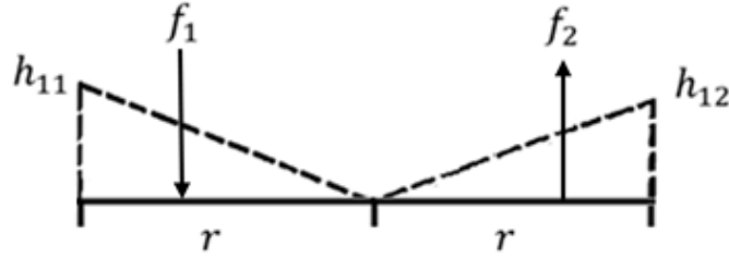
Figure 2-17: Diagram showing distributed loading represented by point loads located at 2/3rds the radius from the tower center (not to scale)
