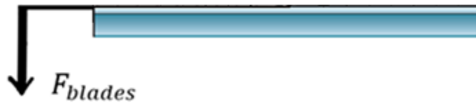
Figure 2-15: Diagram showing the gravity load from the rotor and blades (not to scale)
